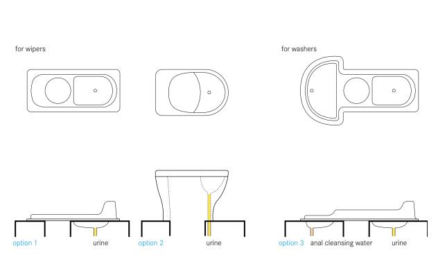
A urine-diverting dry toilet (UDDT) is a toilet that operates without water and has a divider so that the user, with little effort, can divert the urine away from the faeces.
